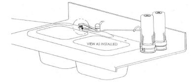
3. □ Turn unit upside down and find the flow indicators "IN" and "OUT" engraved into the plastic near each port. Screw the Plastic Water-In Elbow into the "IN" port & Spout Elbow into the "OUT", insert Spout into Spout Elbow. (If you need to position unit on left side of your sink, switch the wall-mount bracket from front to back of unit, then turn unit around).
