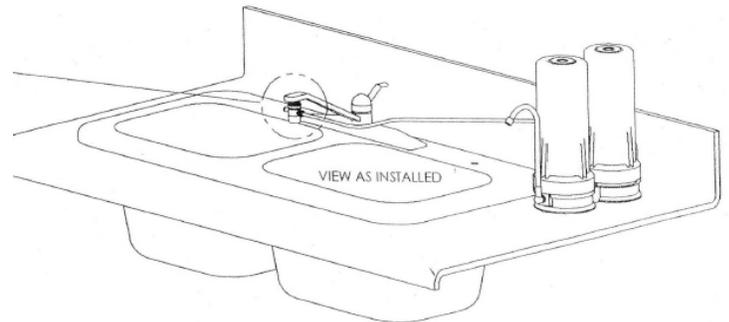
3.  Turn unit upside down and find the flow indicators “IN” and “OUT” engraved into the plastic near each port. Screw the Plastic **Water-In Elbow** into the “IN” port & **Spout Elbow** into the “OUT”, insert **Spout** into **Spout Elbow**. (*If you need to position unit on left side of your sink, switch the wall-mount bracket from front to back of unit, then turn unit around*).
