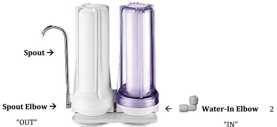
4.  Next, insert one end of the provided **Tubing** into the “**Water In elbow**” until it “pops-in” as far as it can go, then measure how much tubing you will need to comfortably reach the faucet diverter valve and attach to diverter by: unscrewing the metal ring (*off the diverter output*) and putting the tubing through the ring, then attach the tube and screw ring back on to secure. (*Note: make sure to factor in enough “slack” in tubing for when you move your faucet around.*)
