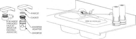
3. Turn unit upside down and find the flow indicators "IN" and "OUT" engraved into the plastic near each port. Screw the Plastic Water-In Elbow into the "IN" port & Spout Elbow into the "OUT" port, then insert Spout into Spout Elbow. (If you need to position unit on left side of your sink, switch the wall-mount bracket from back to front of unit, then turn unit around).
